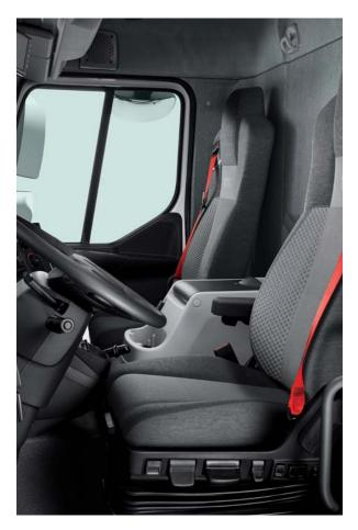
**HEATED PNEUMATIC SEATS** with adjustable side and lumbar supports.
